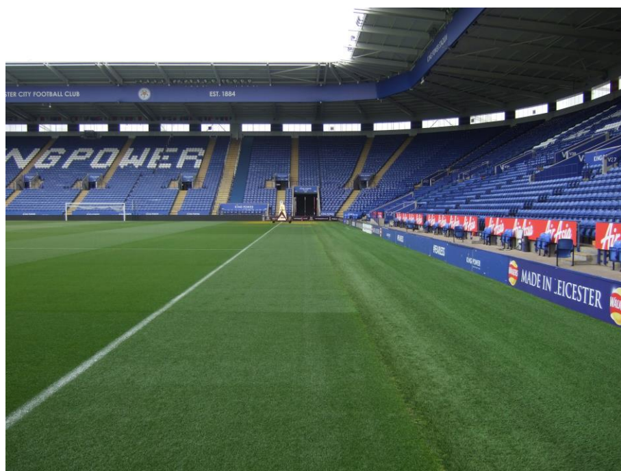
Fig. 14. Ideal scenario of at least 1m of natural turf extending beyond the touchline.
