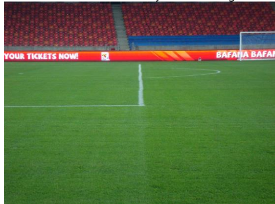
Wavy lines caused by mowing being carried out after line marking.
