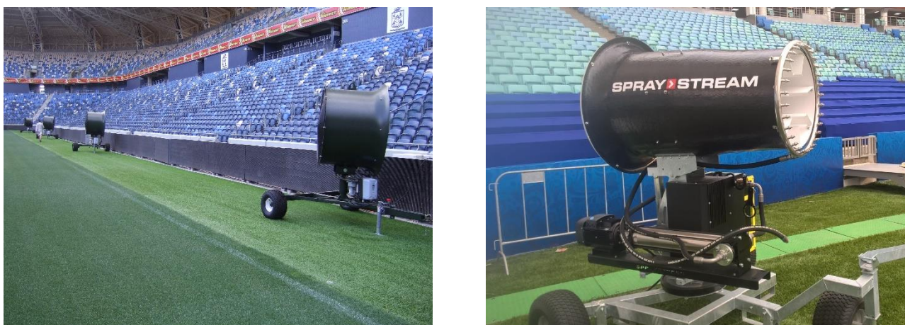
Fig. 11. Examples of pitchside ventilation and cooling fans used to manage turf health.
